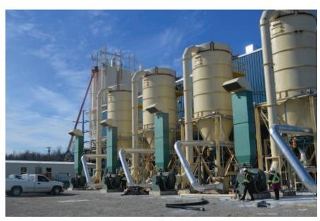
The ORA installed five complete classifier milling systems, each of which included the silo, conveying lines, classifier mill, and all other necessary equipment to process the sorbent.
