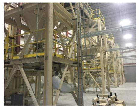
The new system allows ORA to mill and classify the material in one step, ensuring the sorbent is at its most efficient size for the end-user.
